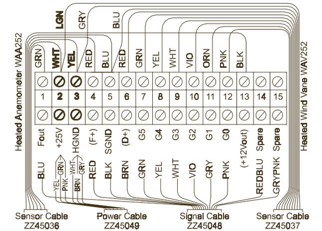
Figure 1. WAC151 Standard Wiring for WAA252 and WAV252
