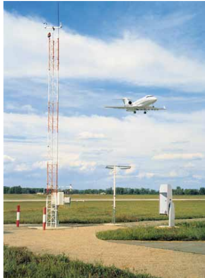
The PWD22 is recommended for Automatic Weather Observation Systems (AWOS).
